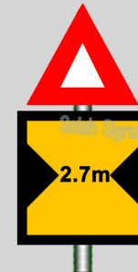
WARNING OF OBSTACLE AHEAD HAVING (A) NARROW (B) LOW CLEARANCE. VEHICLE HAVING GREATER WIDTH OR HEIGHT THAN FIGURE SHOWN UNABLE TO PASS
